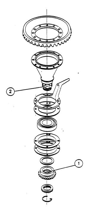
BEVEL GEAR AND FLARED STUB SHAFT ASSY FIGURE 1
