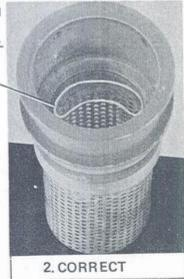
If solder penetration were found insufficient, clean the strainer and solder again (tin soldering).
