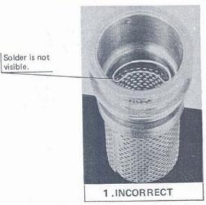
Solder has gone through and blanked off the top holes of the perforated plate.
